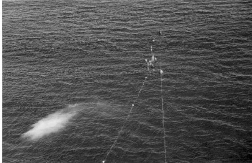
Figure 2. Ebro Delta experiment showing a blob of dye and the velocity measurement station.
