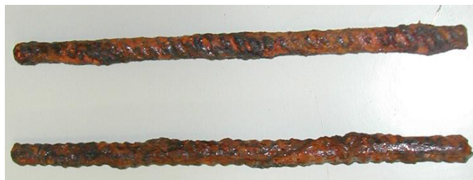
Fig. 3. Specimens after 2016 hours of exposition in the corrosion chamber.
