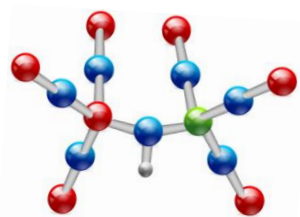
Figure 3.07. Brønsted acid sites in protonic zeolites [blue spheres = O ; green sphere = Al ; red spheres = Si ; white sphere = H ].
