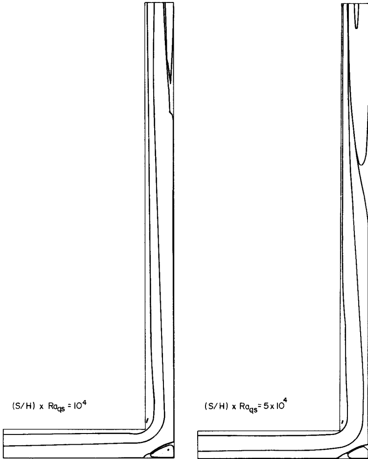
Figure 16. Streamlines for prescribed heat flux. L-shaped channel for S/H = 0.1333 ( S = 0.1 m, H = 0.75 m) and Pr = 0.7 .
