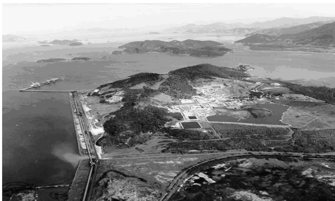
Fig. 1. Tailings of the Zn and Cd smelter at Sepetiba Bay, Rio de Janeiro, SE Brazil in 1996. Note the spill of contaminated material entering the bay after heavy rains. Photo courtesy of C. barcellos.
