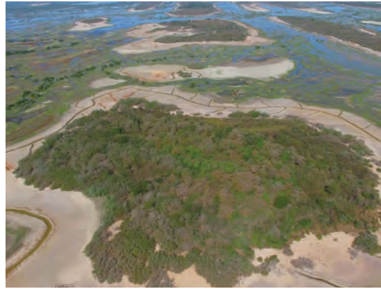
Plain drains: Canals have been installed in this degraded mangrove area to improve water flows, thereby assisting the restoration process. Photo: Ernesto Beltrán García
