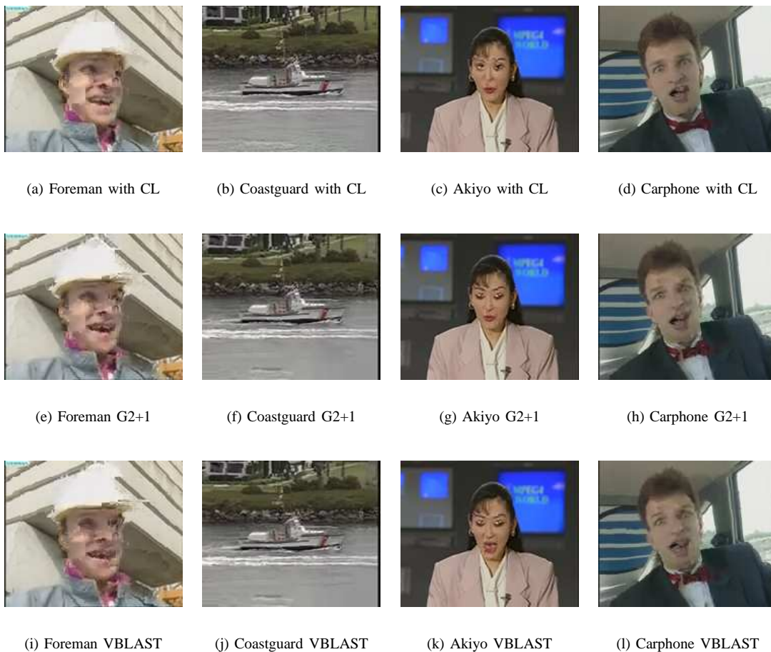
Fig. 4. Subjective quality of the frame 141 in the video sequences transmitted with SNR = 11dB, where frames of the video sequences reconstructed using the algorithm Cross-Layer (CL) appear at the top and the frames with the use of the G2+1 and VBLAST scheme are presented below, respectively.
