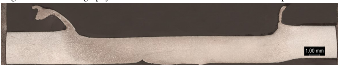
Figure 7.14 – Macrography of Test 6 with 30 kN of axial force and 800 rpm
