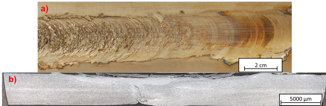
Figure 6.7 – Top (a) and Transverse (b) section for test 5 - 800 rpm, 1 mm/s and 35 kPa
