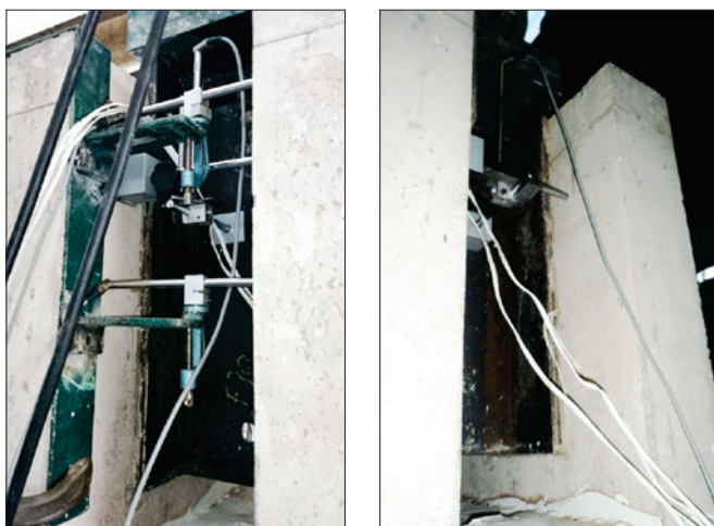
Figure 7 Positioning of horizontal and vertical LVDTs for the push-out tests
