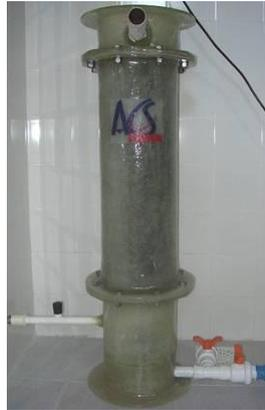
Figura 16 – Reator Aerado Submerso – RAS. LABOSAN - UFC, 2010.
