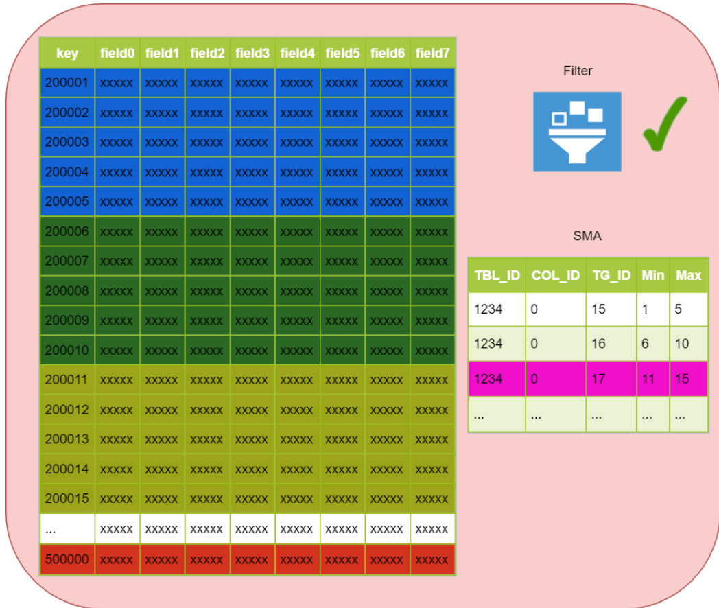
Figure 15 – Filter detection and candidate retrieval
