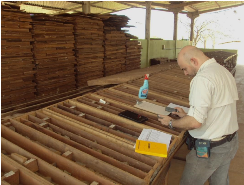
Figure 10 – Description of geological features on drill cores stored in boxes.
